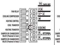
\* If both "Y" and "C" wire are present, tape off "C" wire.
